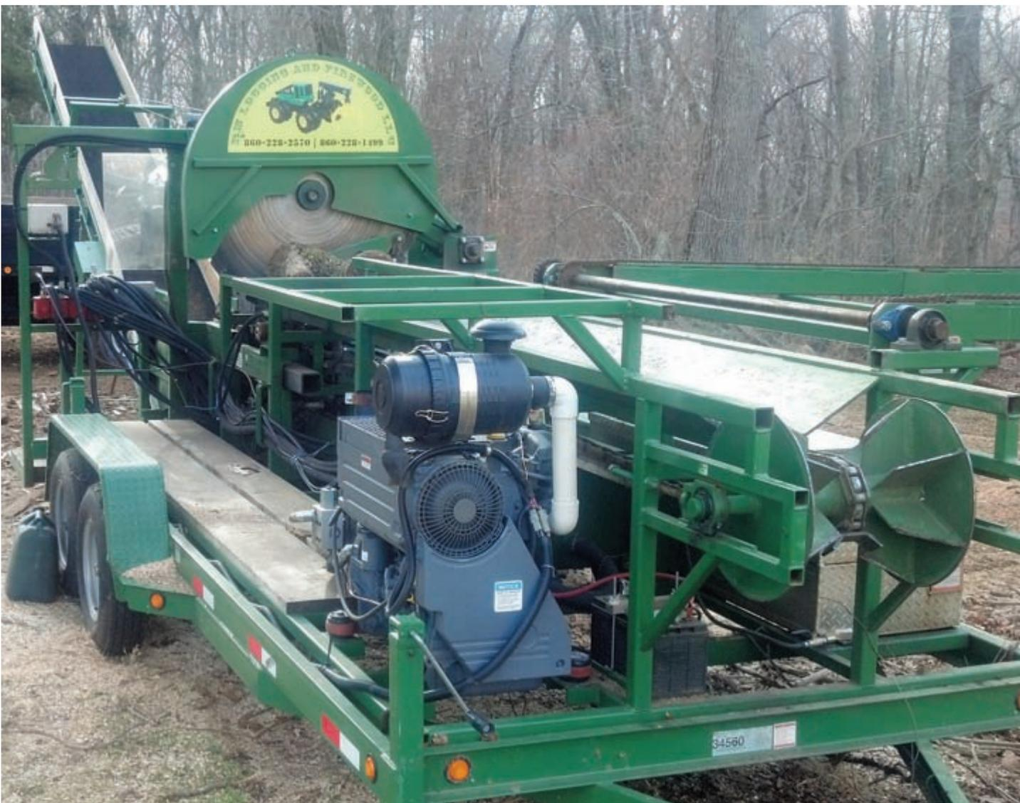
*Messier said, "My Rapido Loco 20 has a live deck that can hold up to a cord of wood. It is easy to setup; I can set it up in less than ten minutes. It has its own conveyor that travels on top of the processor. You can pull the whole shooting match down the road in one shot."*
