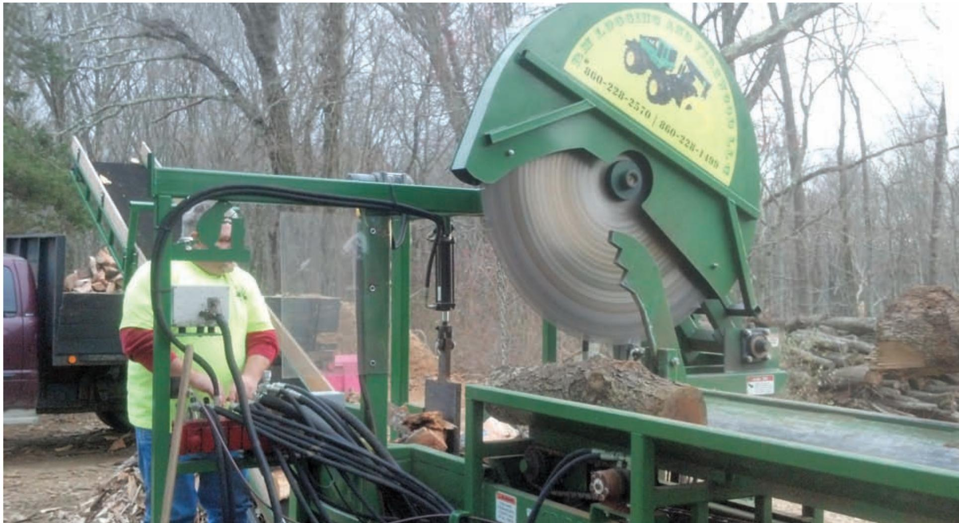
*Woodbine Rapido Loco 20 firewood processor, manufactured by CRD Metalworks, in operation at RM Logging and Firewood.*
