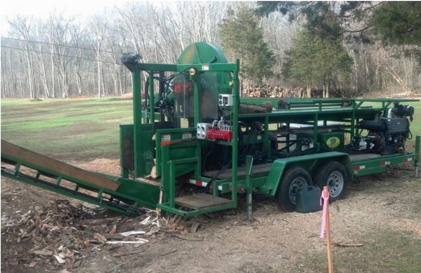
*Cutting and splitting firewood at RM Logging and Firewood on its CRD Rapido Loco 20. This larger machine can process logs up to 20 inches in diameter. Messier said, "I couldn't ask for a better machine. It will push anything through the wedge. It makes a cut in less than half a second."*
