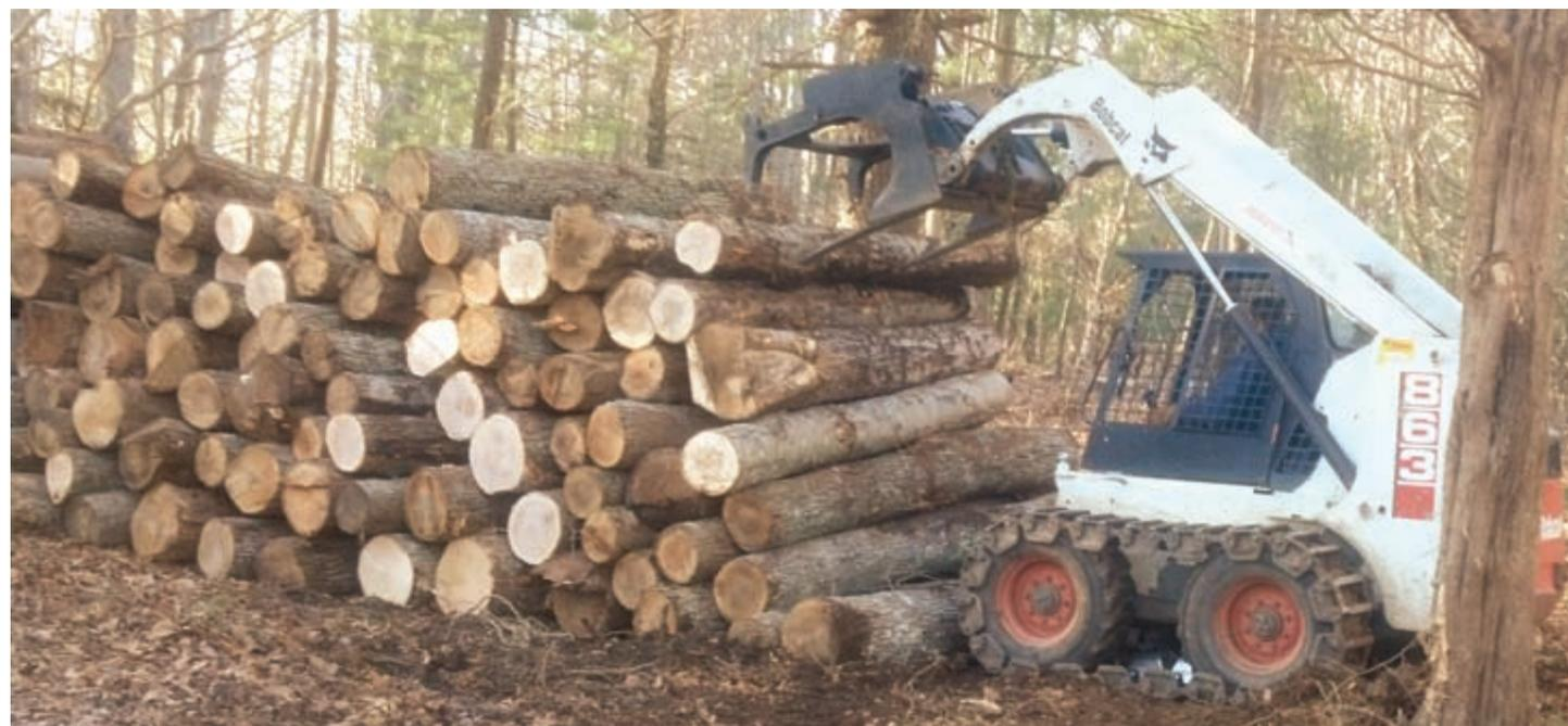
*Loading logs with a Bobcat loader onto RM’s Rapido Loco 20 firewood processor.*
